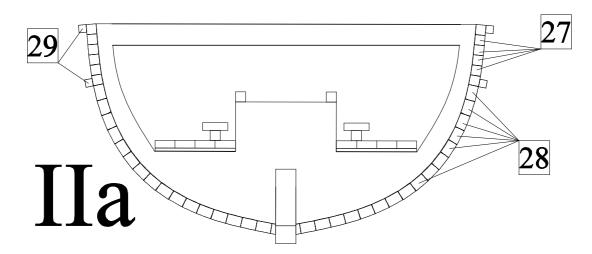
b) After perfect curing of an adhesive cut out upper parts of the frames 5-12.
