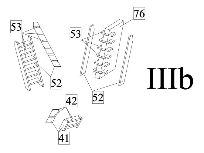
b) Make stairs from parts 41,42 and 52,53. For the production of the stairs use a preparation 76.
