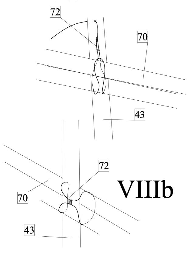
c) Free ends of the ropes for their raising and lowering of the yards tie to beams 46. To the ends of the yards tie ropes 72 for controlling of yard elevation and the free ends of the ropes tie to beams 46. A scheme of the running rigging is shown in 1:2 scale in the plan 3B.
