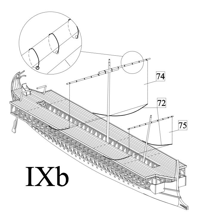
c) To a lower edge of the sails tie ropes 72 for raising and lowering of sails. Then run the ropes around yards and tie them to beams 46. A scheme of the sails is shown in 1:2 scale in the plan 3C.
