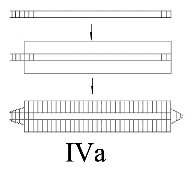
b) First glue beams 48 to the longitudinal beams 37. Then glue the skeleton of the upper deck to the beams 48. Then glue also rest of beams 48 and 46 to the construction. Finally reinforce the construction by reinforcement beams 51.
