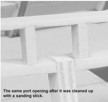
ing looks like after it was cleaned up with a sanding stick. There will be a need to repeat this process for another port opening on the gun deck as well.
