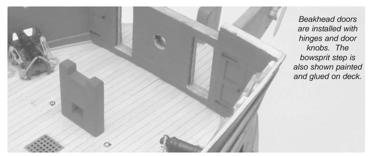
between the uprights. You can use as many of these packing pieces you need as long as the angle of the opening matches the plans when you are done. To finish it up, add two more strips along the inside edge of each upright so the opening is the correct width. Paint the bowsprit step red when you're done. See the photos provided.
