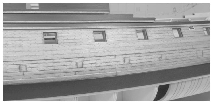
cast scrollwork. These will be positioned as a continuation of the molding, so try and match the profile as closely as possible. Examine the plans carefully to see where the molding is positioned. Note how the molding terminates in the waist with the scrollwork.
