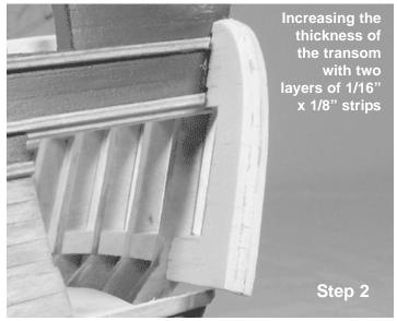
adjust the spacing between your lintels and sills if you need to so they match the opening created by the laser cut transom. See the photo provided. Once the transom is in position, you can cut and glue the uprights (1/16" x 1/8" strips) onto the outboard side of each stern timber to finish it off.
