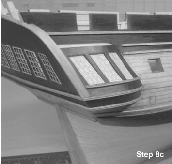
the top of piece QG4 after the glue dries. See the photo for step 8 that shows this first layer glued in position. You should stain the inboard side of this first layer before you glue it onto the model permanently. It will be very difficult to do afterwards.
