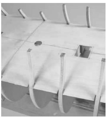
the slots along the edge of each piece if needed. Note: The two sections of the false decking for the port side should meet along bulkhead #1. They should share the top of the bulkhead edge.
