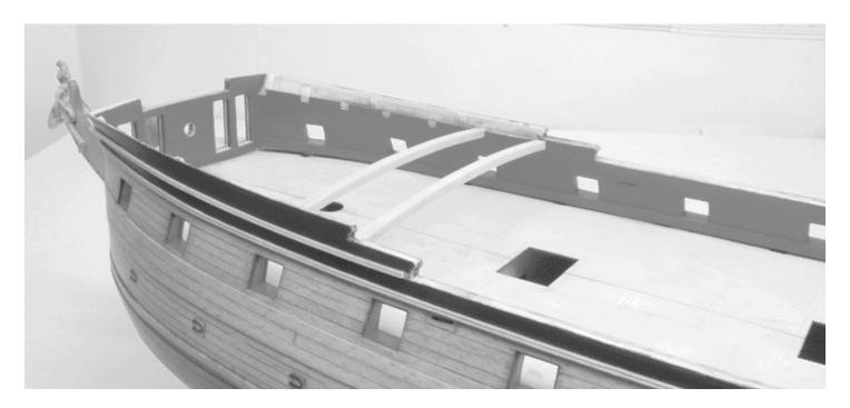
being, glue a  $\frac{1}{3}$ " x  $\frac{1}{32}$ " strip on top of the first layer of spirketting you added in step one. Be sure to align the top of this second layer with the top of each gun port sill just like you did for the first layer. Soften the top edge of the spirketting so it doesn't have a hard edge. Just run some sand paper down the top of it to knock off/round off the sharp edge.
