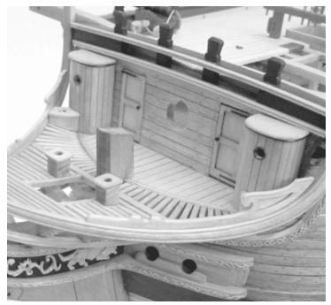
how two small openings were framed for the seats of ease. See the photo provided that shows the head grating completed. The forward-most beam will be a 3/32" x 3/32" basswood strip. You can see this featured on sheet one of the plans.
