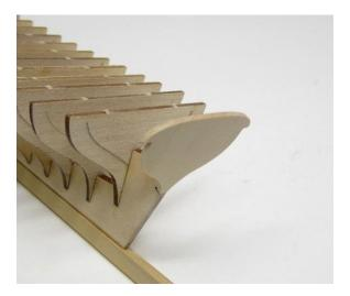
important as the hull will not be faired properly if they are not lined up. You should view the bulkheads from above to make sure they are glued in at a right angle to the keel and spaced evenly apart as well. You might consider using yellow wood glue for this because the open time is longer. This will give you more time to make adjustments before the glue sets permanently.
