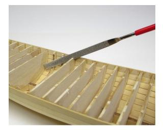
Basically you have to cut through the top of each bulkhead down to the laser cut line on each side. Then bend the center so it snaps off at the base. I recommend using a needle file as shown in the photo. I had tried using a mini razor saw, but it pulled too much and split the wood along the top of the frames. Use a gentle stroke and don't apply too much pressure.
