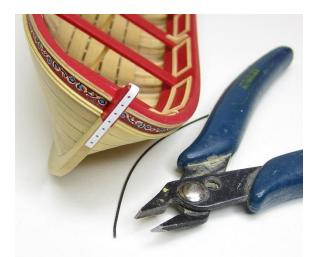
slightly proud of the surface so it would simulate a bolt head. This is a feature that can be seen on most contemporary models of barges and pinnaces.
