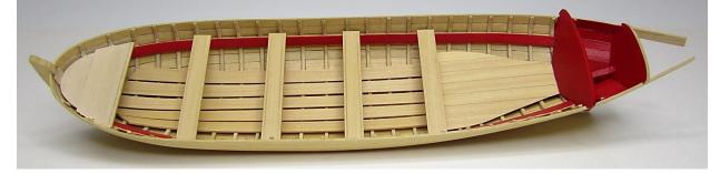
sure it fit properly, I cut the platform to shape and glued it into position. Then I glued the first thwart on the model. The thwart actually butts against the platform and sits flush with it. Also note in the photo posted on the previous page that the seatback and helmsman area were painted red before the thwarts were added.
