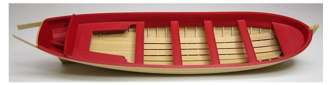
to fill any gaps. The thickness of the hull along the sheer was just 3/32" after sanding the planking inboard and outboard. It was sanded to create a uniform thickness from bow to stern. The photo on the top of the previous page shows the planked bulwarks. The interior planking was painted red afterwards.
