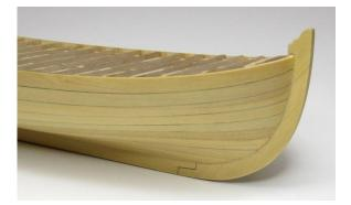
be consistent at all. In all probability, it will be wider than 3/16" (especially at mid-ship). A wider 1/4" x 1/32" strip is provided in the kit for this purpose. Carefully shape this final plank to fit the opening on your hull. Because it is in the middle of the hull where it begins curving towards the keel, the wider plank won't be noticeable when viewing the model from port or starboard.
