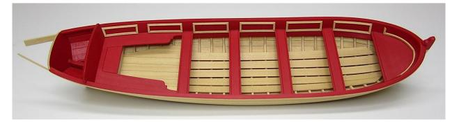
place. Use light passes at first and then several heavier passes as the profile develops. It will take many passes along the edge to develop the fancy edge. Take your time here. If, for whatever reason, the cap rail doesn't look right or the wood becomes damaged, just pop off the cap rail and replace it.
